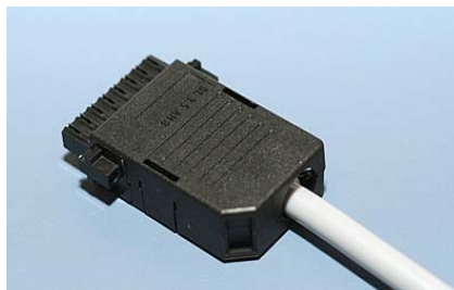
Fix the upper part of the strain relief housing by snapping it onto the lower part.
